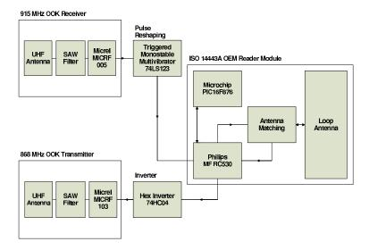
Fig. 3. Hardware diagram of the Mole
