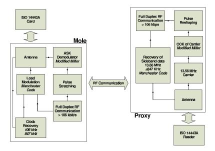
Fig. 1. Functional analysis of the relay system
